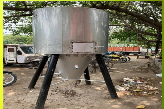
SOLID WASTE INCINERATOR
